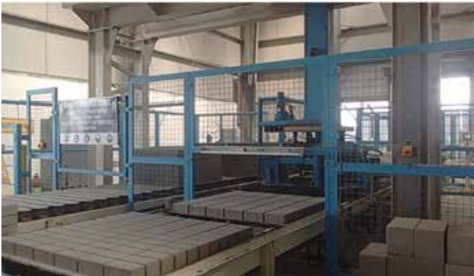
A block-making trial using LC3
