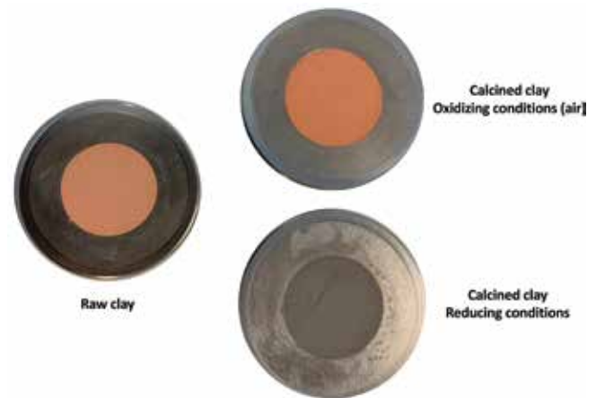
Color appearance of raw and calcined clays obtained with and without use of color control procedures during the cooling process (from Reference 2)
