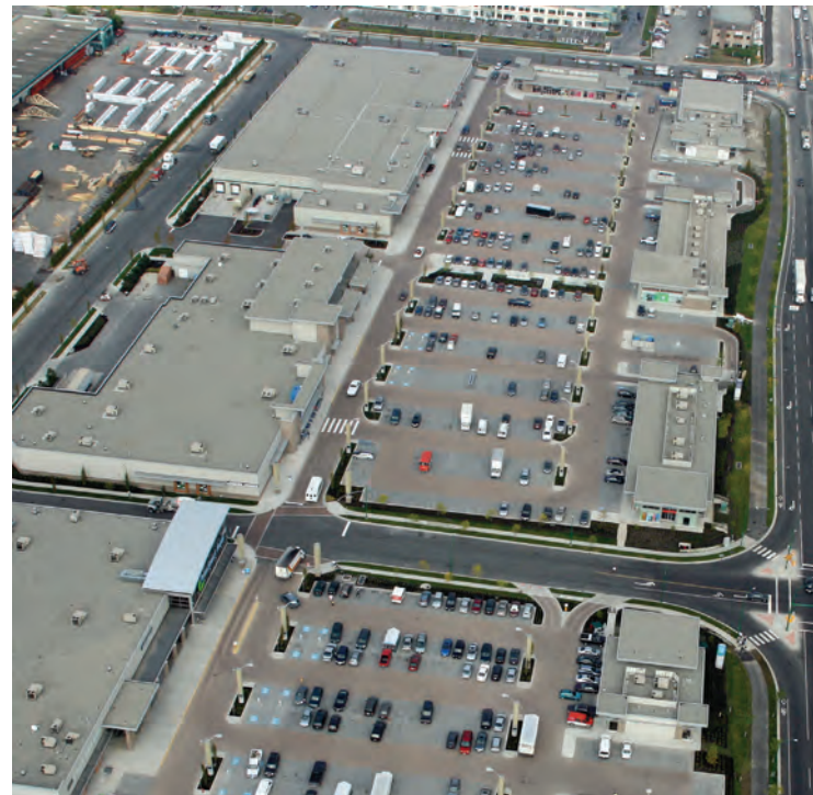
Fig. 3.38—With no space for a separate detention pond, the permeable interlocking concrete pavement parking lot becomes the detention facility for roof and parking lot runoff. Photo courtesy of Interlocking Concrete Pavement Institute
