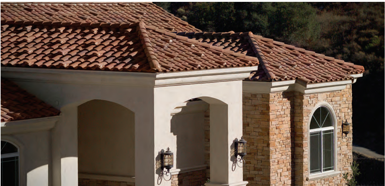
Fig. 3.80—Concrete roof tiles are available in various shapes, sizes, and colors and provide protection against large hail, wind, fire, and other aggressive conditions. Photo courtesy of Tile Roof Institute
