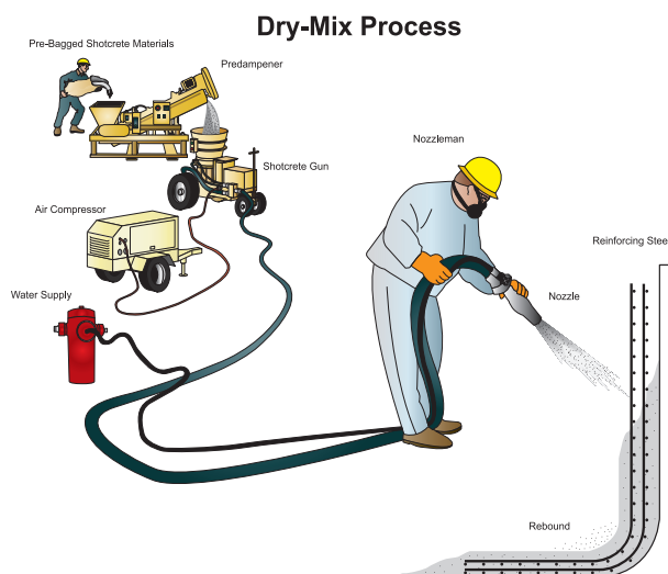
Fig. 3.78—Dry-mix shotcrete process. The dry mixture is conveyed pneumatically through the delivery hose, and water is added at the end nozzle. Photo courtesy of American Shotcrete Association
