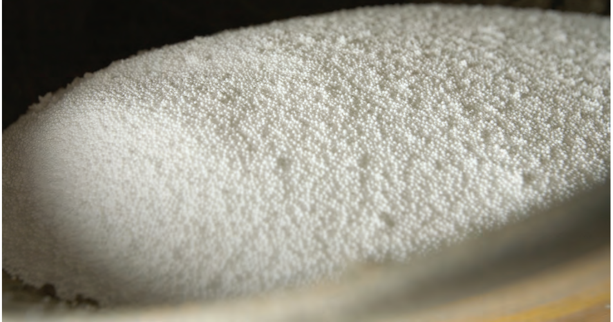
Fig. 1.30—A loose pile of Elemix® XE concrete additive. Photo courtesy of Syntheon, Inc.
